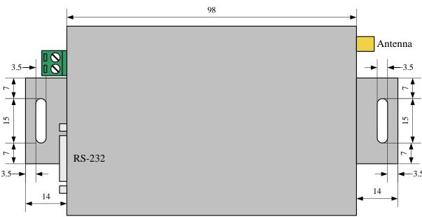
Side (the side of the antenna) dimension shown as below: (Unit: mm)
